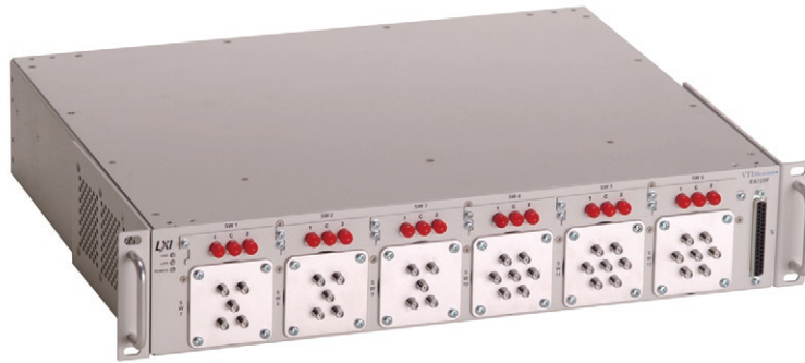
EX72SF with 6 multi-throw and 6 SPDT 26.5 GHz relays
