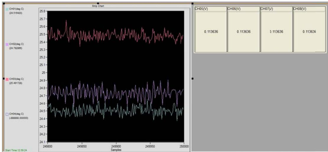
Monitoring temperature and voltage data in **Acquisition Display**
