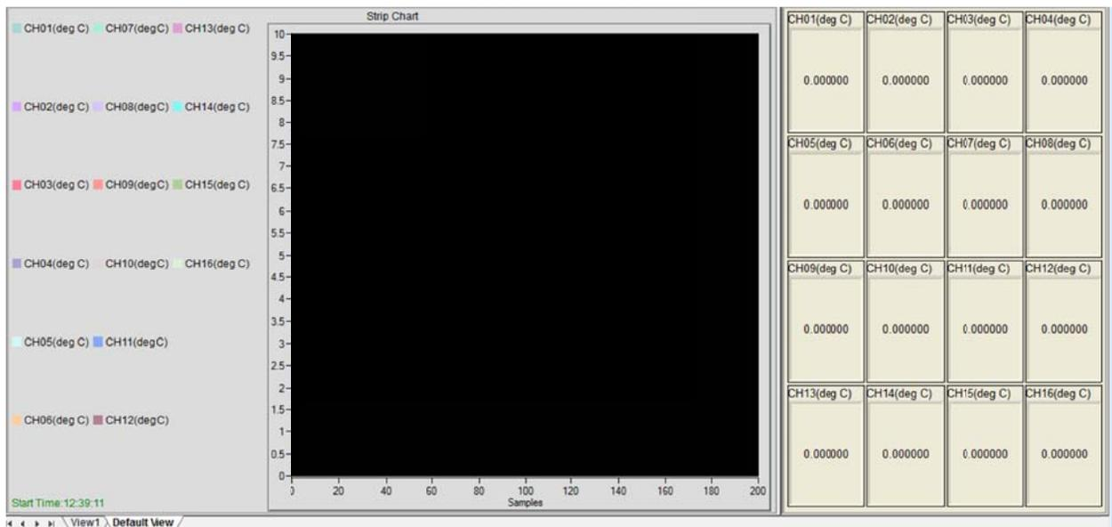
The **Default View** shows all 16 channels in a **Strip Chart** and a **Digital Readout** display. This allows any user who uses all 16 channels to acquire and monitor data instantly from all 16 channels without the need of setting up the data displays prior to the data acquisition process. However, in this example, not all 16 channels are used so a new view needs to be created.
